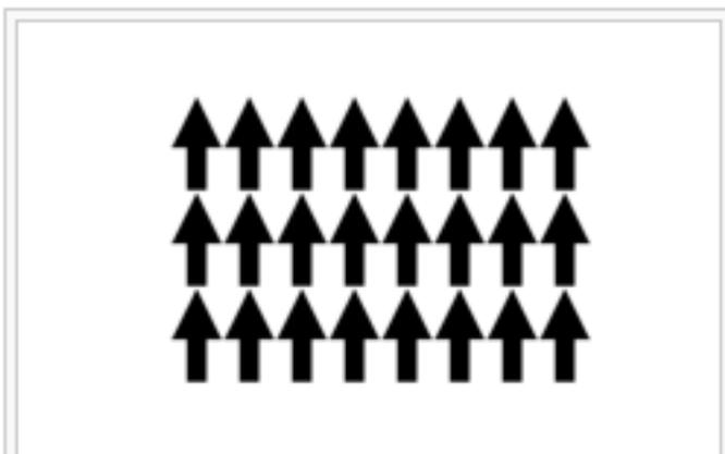
**Figure 1** Below the Curie temperature, neighbouring magnetic spins align in a ferromagnet in the absence of an applied magnetic field.
