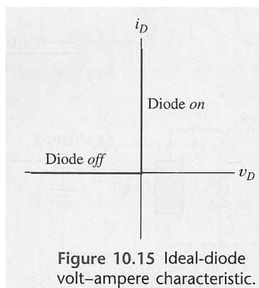
Figure 10.15 Ideal-diode volt-ampere characteristic.
