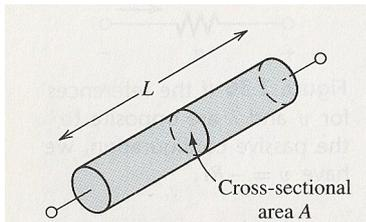
**Figure 1.38** Resistors often take the form of a long cylinder (or bar) in which current enters one end and flows along the length.
