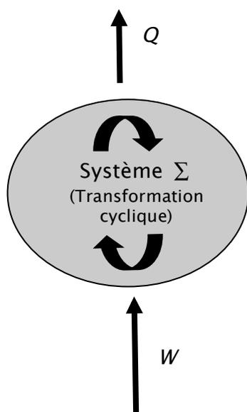
1<sup>er</sup> principe:  $\underbrace{\Delta U = 0}_{\text{car cyclique}} = W + Q$
