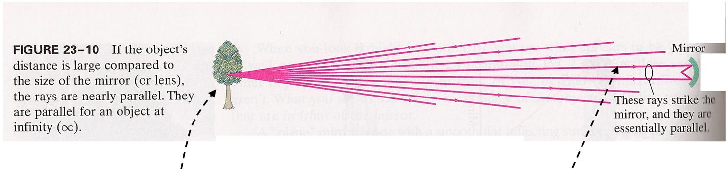
**FIGURE 23-10** If the object's distance is large compared to the size of the mirror (or lens), the rays are nearly parallel. They are parallel for an object at infinity ( $\infty$ ).
